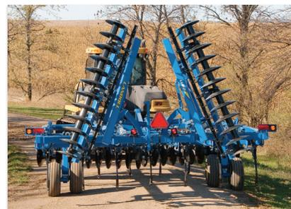
2211-13 and 15 shank models feature folding rear gangs for reduced transport width. Transport height on 13 and 15 shank folding models; 13' 4" & 14' 0" respectively.
